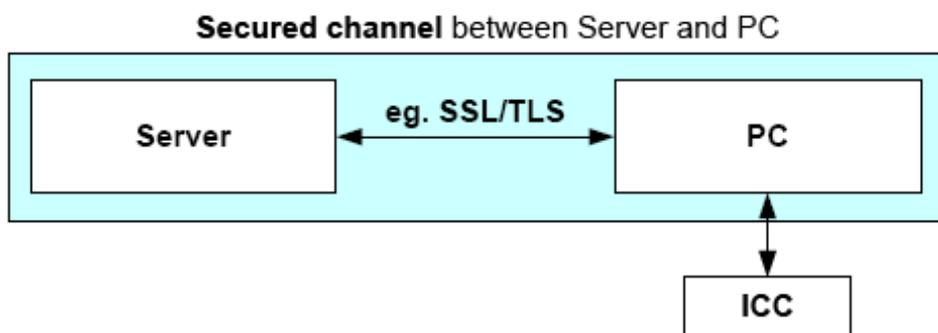
In the above example (taken from EN 419212-2), client/server authentication establishes a secured channel between a remote server and a PC. The ICC will be used as a cryptographic toolbox in order to provide the cryptographic functionality to the PC. If a process needs a certificate from the card that is not provided by OpenPGP (e. g. x.509), then it can be stored in the DO 'Cardholder certificate' (7F21 AUT) as 1st occurrence.
